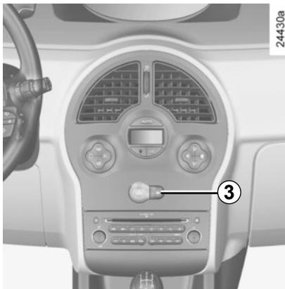
To lock the vehicle leaving a door open (eg. when transporting something in the luggage compartment which prevents it from being closed), or when the vehicle is located in a zone of high electromagnetic radiation, or if the card or key is faulty: with the engine switched off, press and hold button **3** for more than five seconds.
