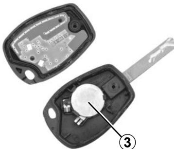
**Note:** It is not advisable to touch the electrical circuit in the key cover when replacing the battery.
