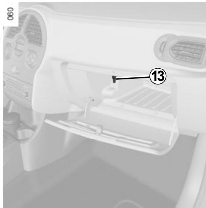
Depending on the vehicle, this glove box compartment is ventilated and air conditioned in the same way as the passenger compartment.
