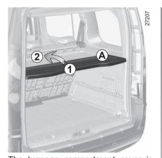
The luggage compartment cover is made up of two rigid sections.
