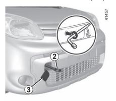
Only use the front and rear towing points (never use the driveshafts). These towing points may only be used for towing: never use them for lifting the vehicle directly or indirectly.
