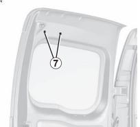
Remove the two plastic blanking covers **7** from the inside. Unclip the light using a screwdriver, by pressing in the metal clip housings.
