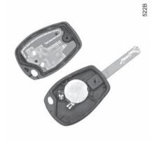
**Note:** it is not advisable to touch the electronic circuit in the key cover when replacing the battery.
