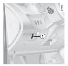
Control knob 1 is used to adjust the height of the headlight beams according to the load.
