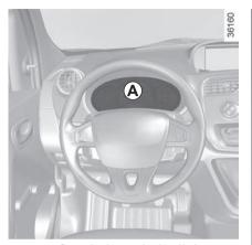
Seat belt reminder light Depending on the vehicle, it is displayed on the instrument panel or on the central display of the dashboard. It remains on when the engine is started if your seat belt is not fastened. A beep sounds at a low volume for 30 seconds. then at a high volume for 90 seconds.
