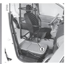
Pivot the moving section 90 degrees, lock it at point 5 and lower catch 3.
