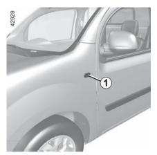
Unclip indicator light **1** on the door side, using a flat-blade screwdriver type tool.
