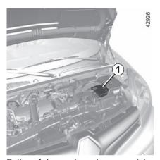
Battery 1 does not require any maintenance. You should not open it or add any fluid.
